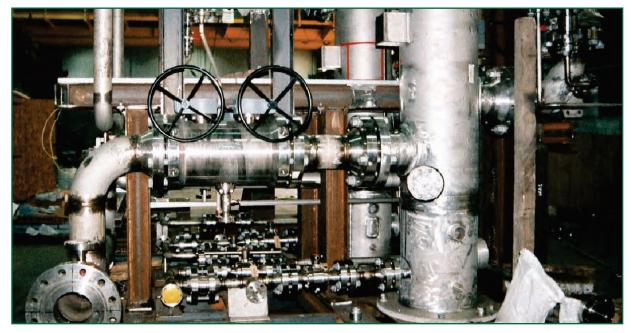
Skid package footprint reduced therefore skid cost reduced by keeping the valve envelope to standard ASME B16.10 length.
