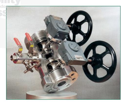
Looking at a traditional hook up, two traditional single 3 piece isolate ball valves and spool piece means a potential of, 8 additional leak points (2 from trunnion, 4 from 3 piece design, 2 from spool joints.) Compared to one piece Twinsafe with slipper plate trunnion design.
